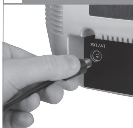
Plug the coaxial cable of the antenna into the TV input socket
