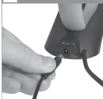
Connect the AC adaptor to electric mains, and the output wire plug into the DC input socket of the antenna
